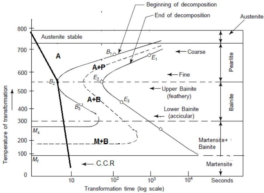
Fig. 4: TTT diagram for eutectoid steel
