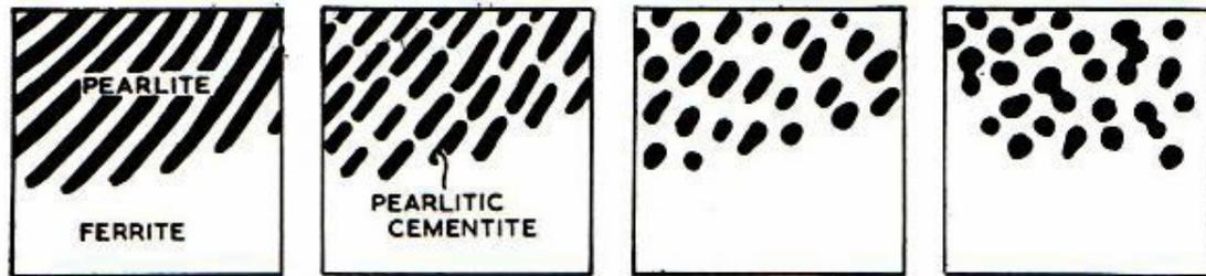
Figure 3. The Spheroidisation.
