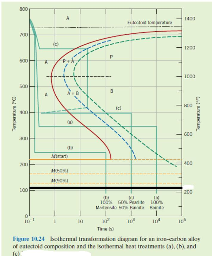
Figure 10.24 Isothermal transformation diagram for an iron-carbon alloy of eutectoid composition and the isothermal heat treatments (a), (b), and (c).
