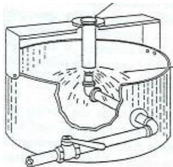
Fig.1 Schematic illustration of the Jominy end-quench test
