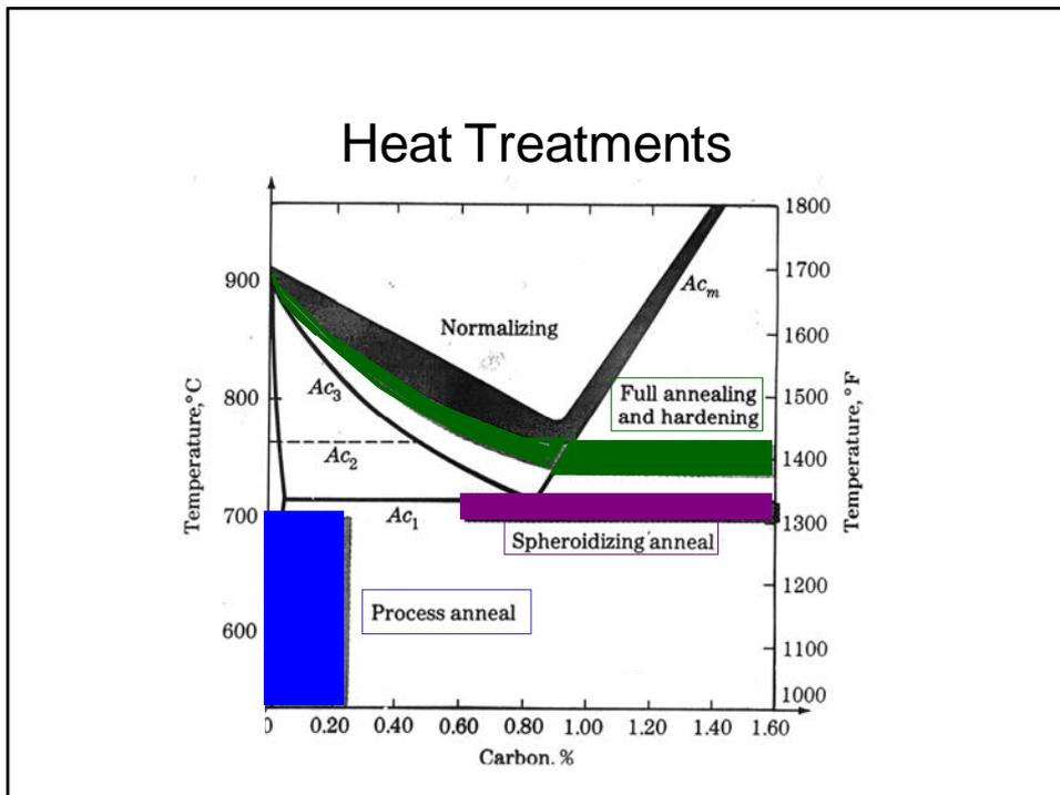
Figure 1. Heat-treatment temperature Ranges of Classes of Carbon Steels.
