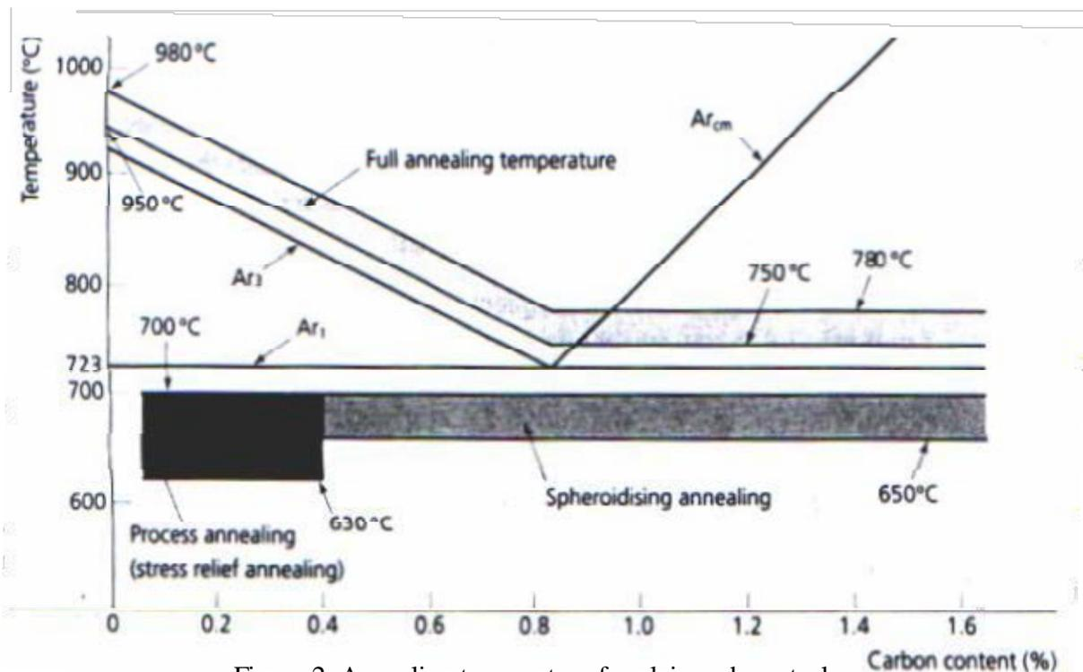
Figure 2. Annealing temperature for plain carbon steel .
